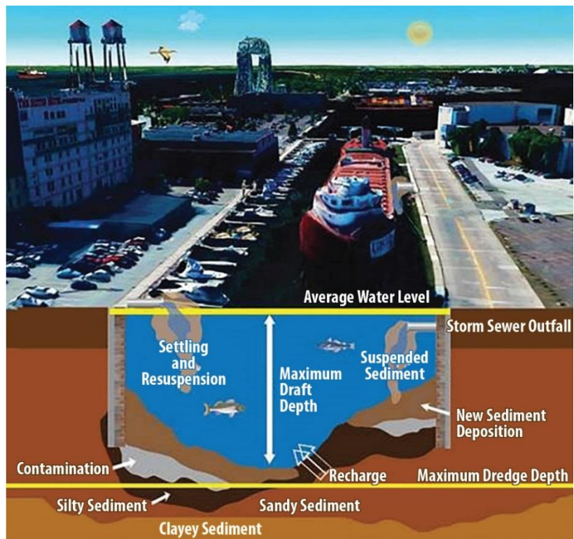
Photo of Minnesota Slip in Port of Duluth-Superior with a cross-section diagram displaying the current sediment issues.
