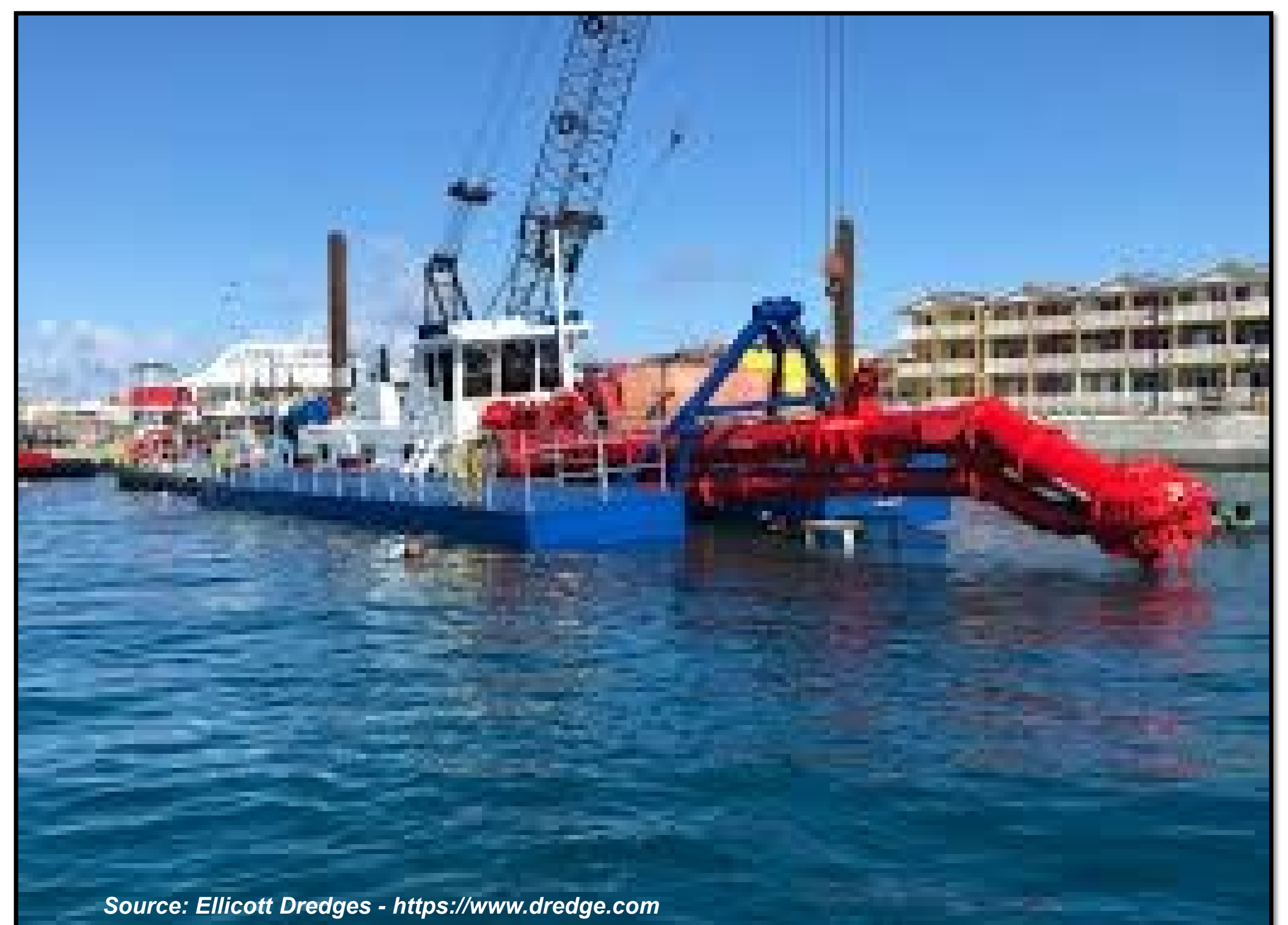
Cutterhead attached to dredge pipe.
