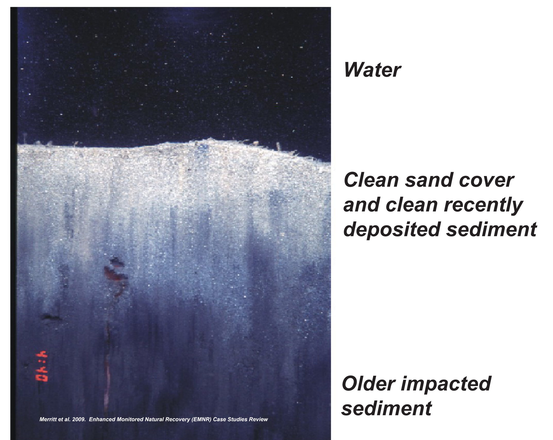
Conceptual example of ENR sediment cover.
