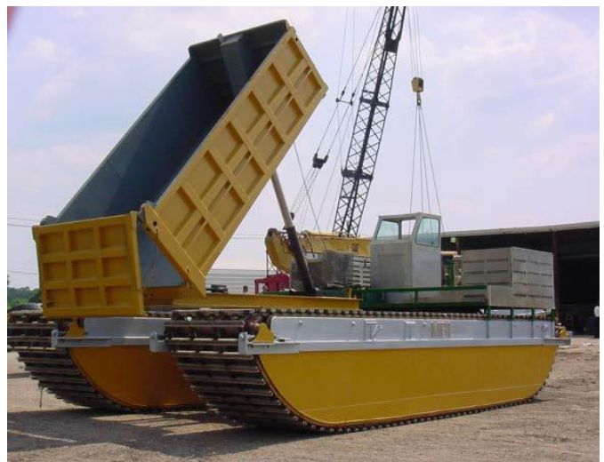
Marsh buggy dump truck used to move excavated material and fill marsh.
