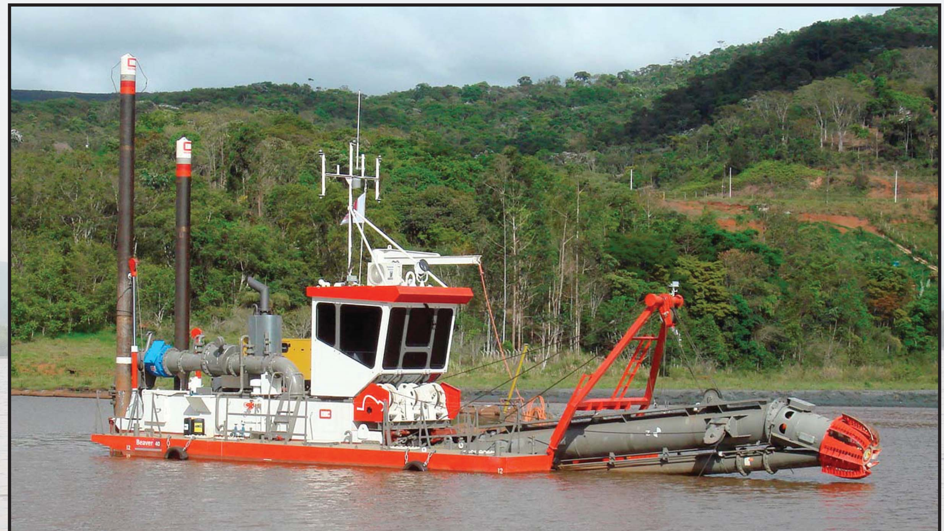
Hydraulic dredge with cutter above water
