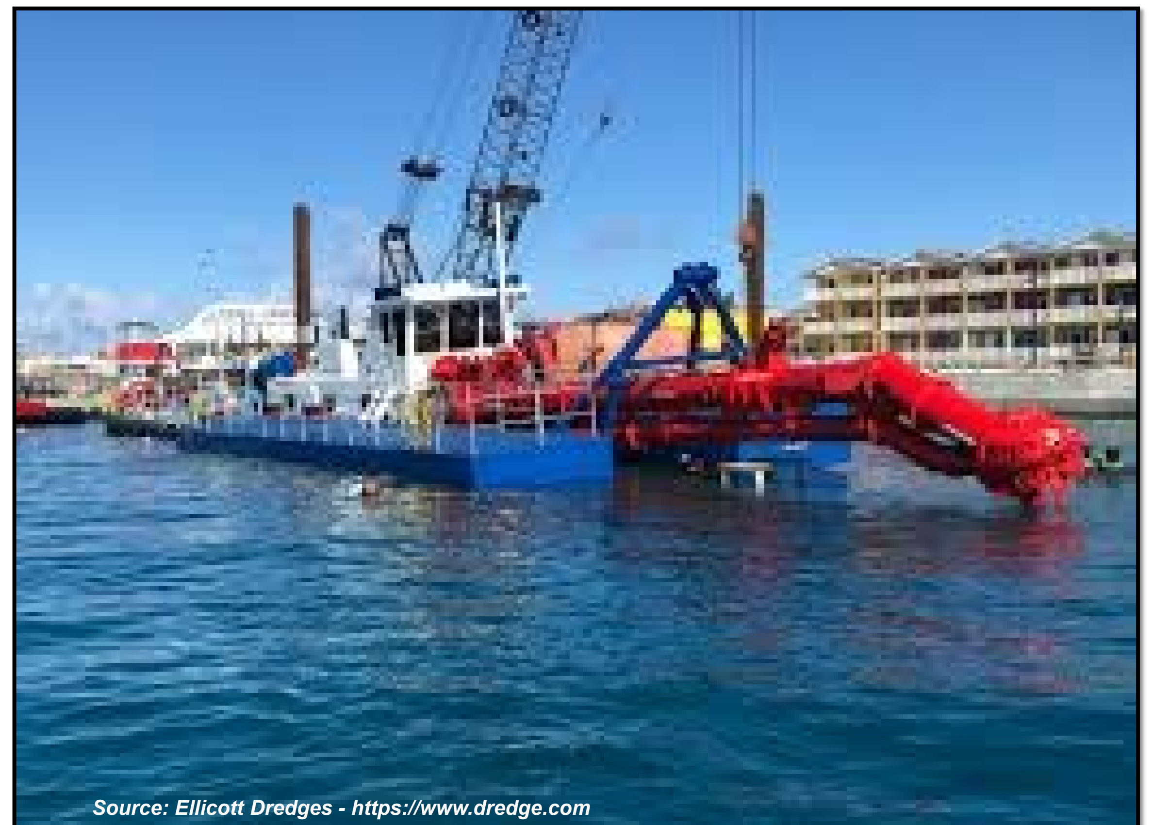
Cutterhead attached to dredge pipe.
