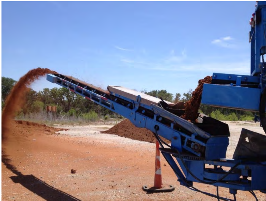
Photo showing stone slinger equipment; photo from http://bcginvestments.net/Stone_Slinger.html
