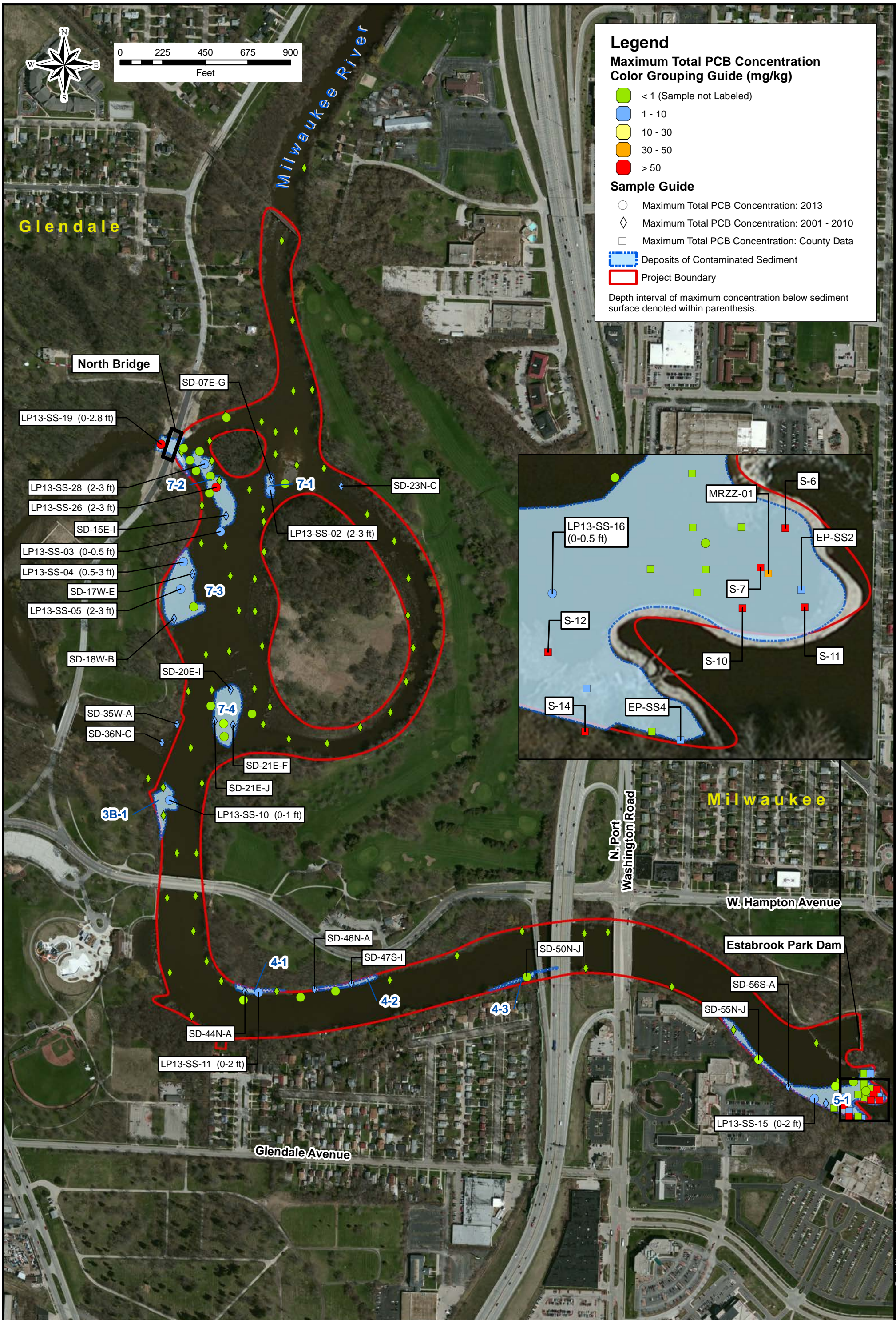
Figure 2-2 Total PCB Concentrations Detected in the Phase II Area of the Lincoln Park/Milwaukee River Channel Sediments Site
