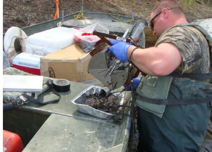
Removal of sample from ponar device.
