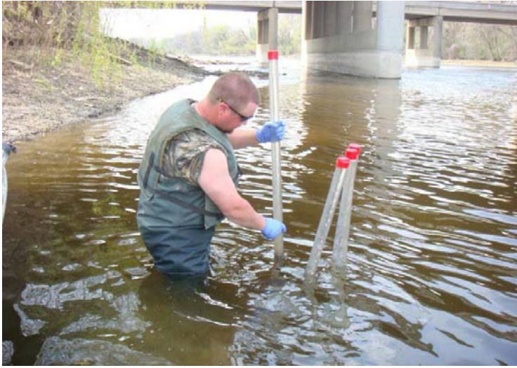
Lexane manually removed sediment and measured for recovery.
