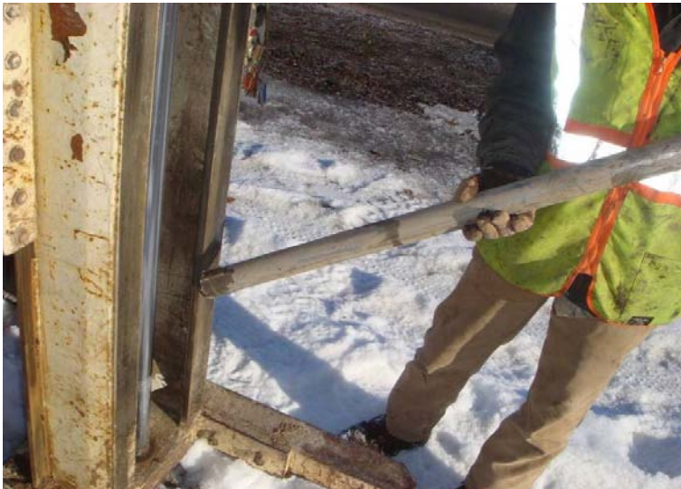
Discrete sampler can be driven to desired depth, opened, and then driven up to 5ft for sample collection into acetate sleeve.
