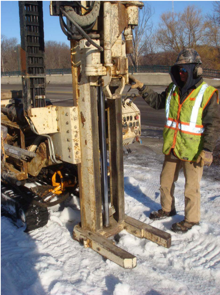
ATV-mounted Geoprobe rig used for sediment probing and core collection
