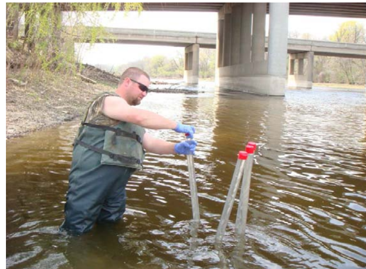
Lexane is capped to create vacuum to hold sediment in.
