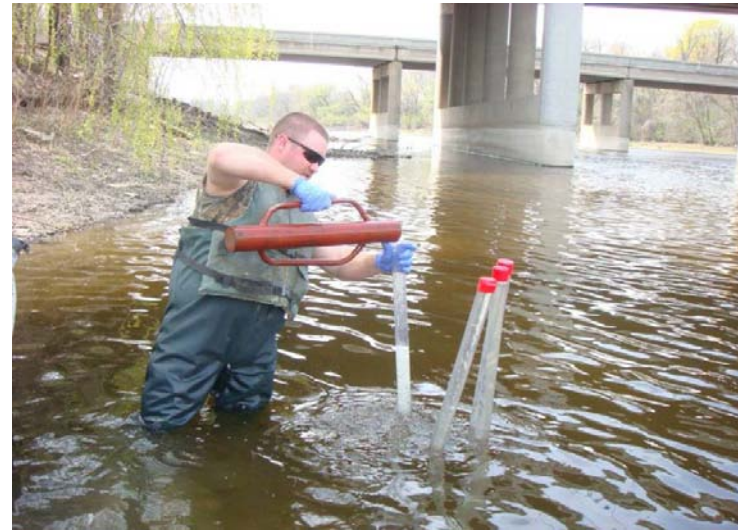
Lexan core tubes used for manual core collection. Once driven to refusal, they are filled with water and capped to create vacuum.
