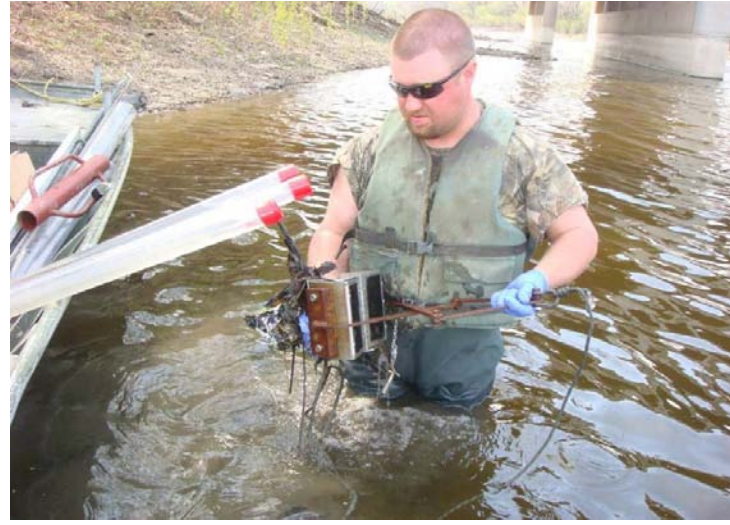
Retrieval of sediment sample using ponar device.
