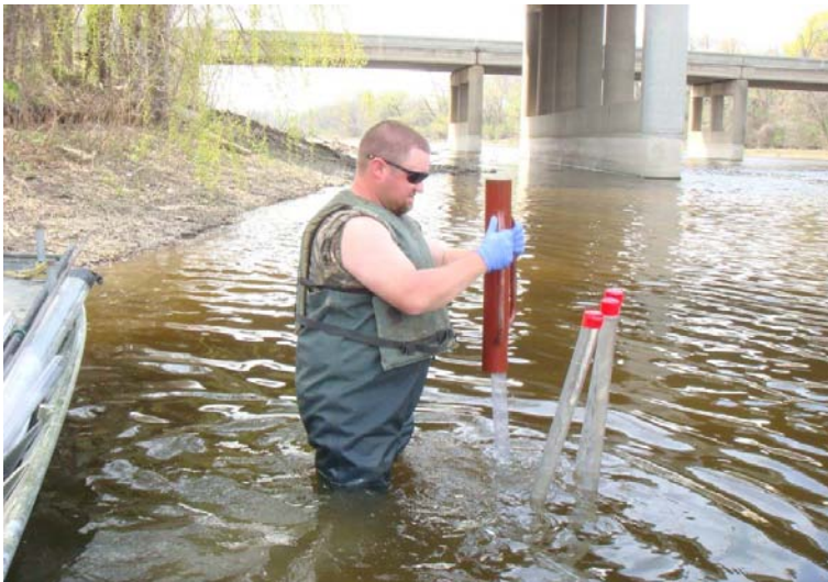
Lexane is driven to desired depth or refusal using a fence post driver.
