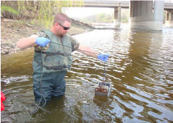
Ponar samples were collected for 0.0-0.5' interval.
