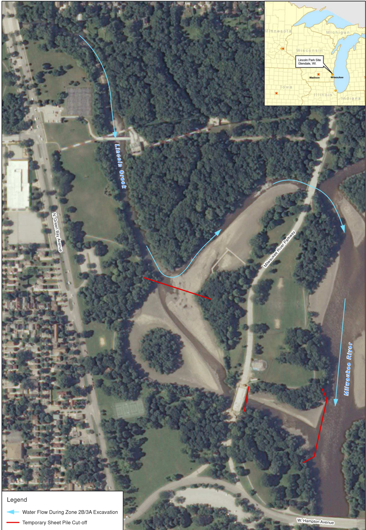
Figure 2b Stage 2 Temporary Cut-off Lincoln Park/Milwaukee River Site Glendale, WI
