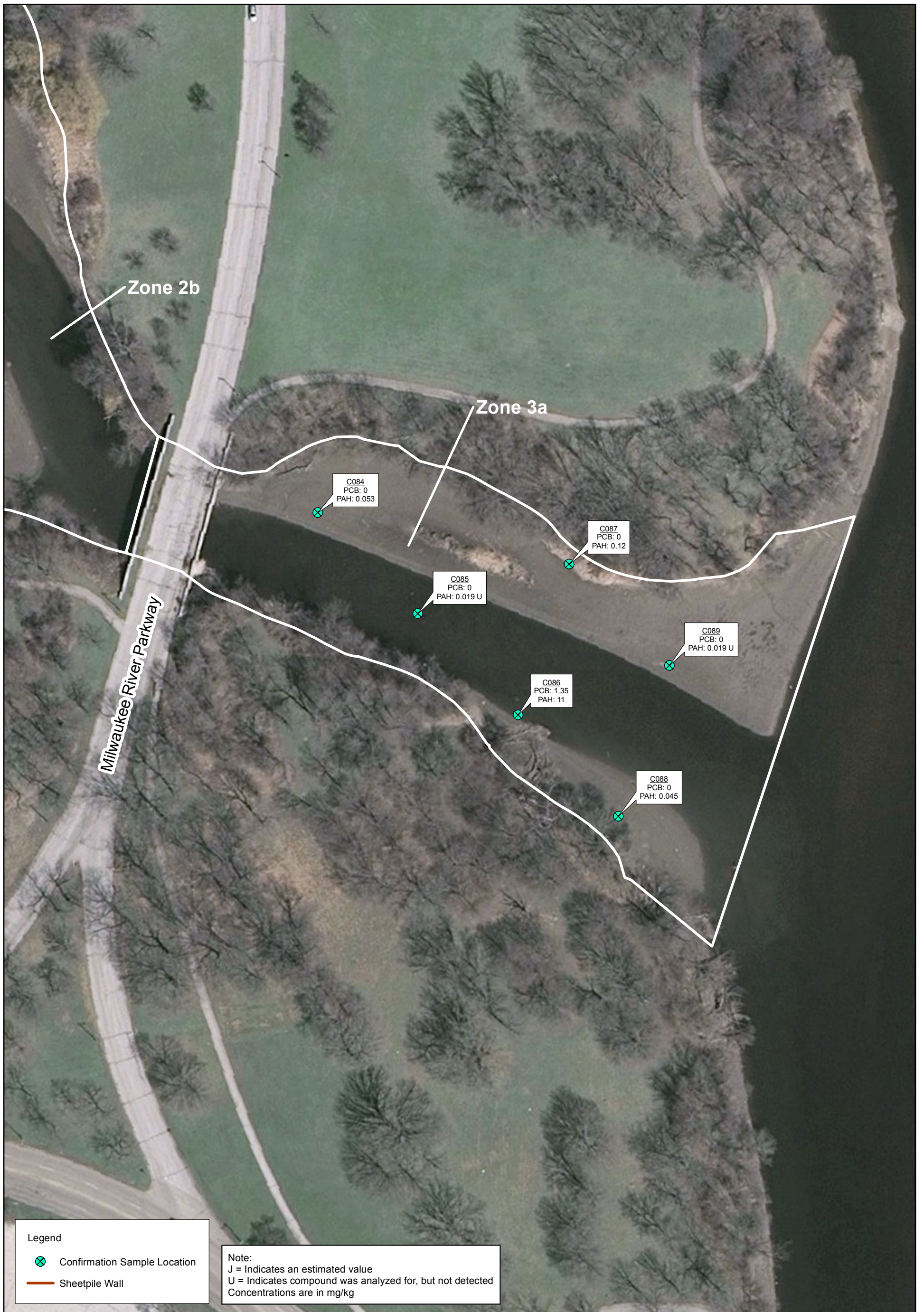
Figure F-4 Final Surface Concentrations - Zone 3a Filed Sampling Plan Glendale, WI
