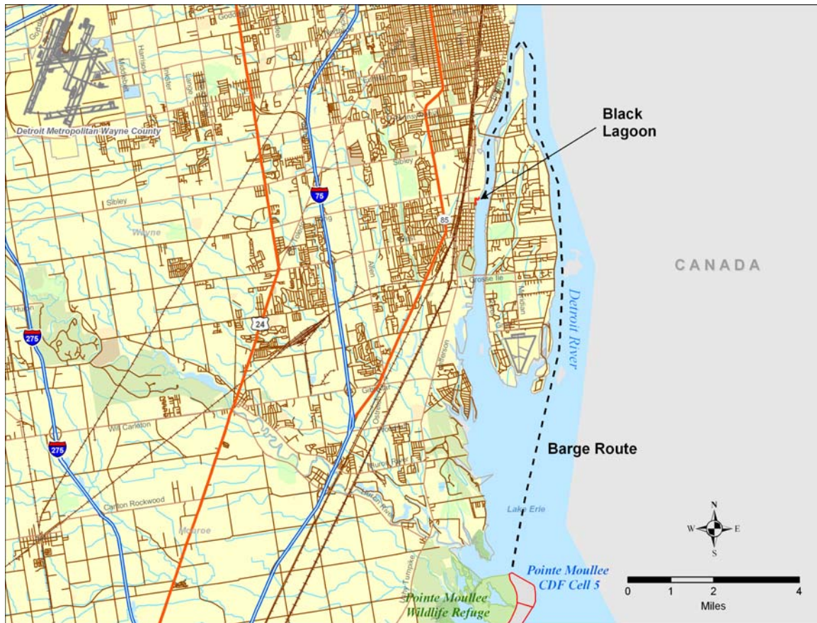
Figure 3-2 Map of Detroit Area With Barge Route From Black Lagoon to the Pointe Moullée CDF
